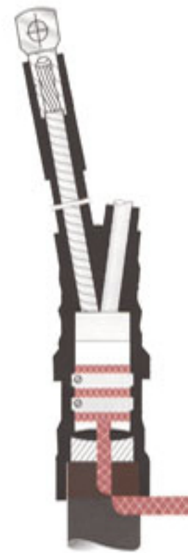
1.1 kV PILC Termination
